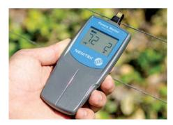
The Nemtek Fence Meter helps diagnose problems on your fence to optimise the electric fence installation and ensure that the fence operates at an ideal level.
