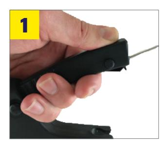
Flick the tagger pin out horizontally and hold your thumb down on the top arm of the tagger. This locks the tagger pin into position.
