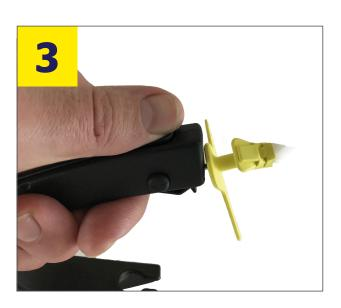
Push the rest of the tag onto the tagger pin.
