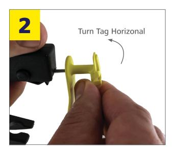
Gently slide the tag onto the tagger pin until you feel the tagger pin touch the end of the tag. Straighten the tag's surgical tip.
