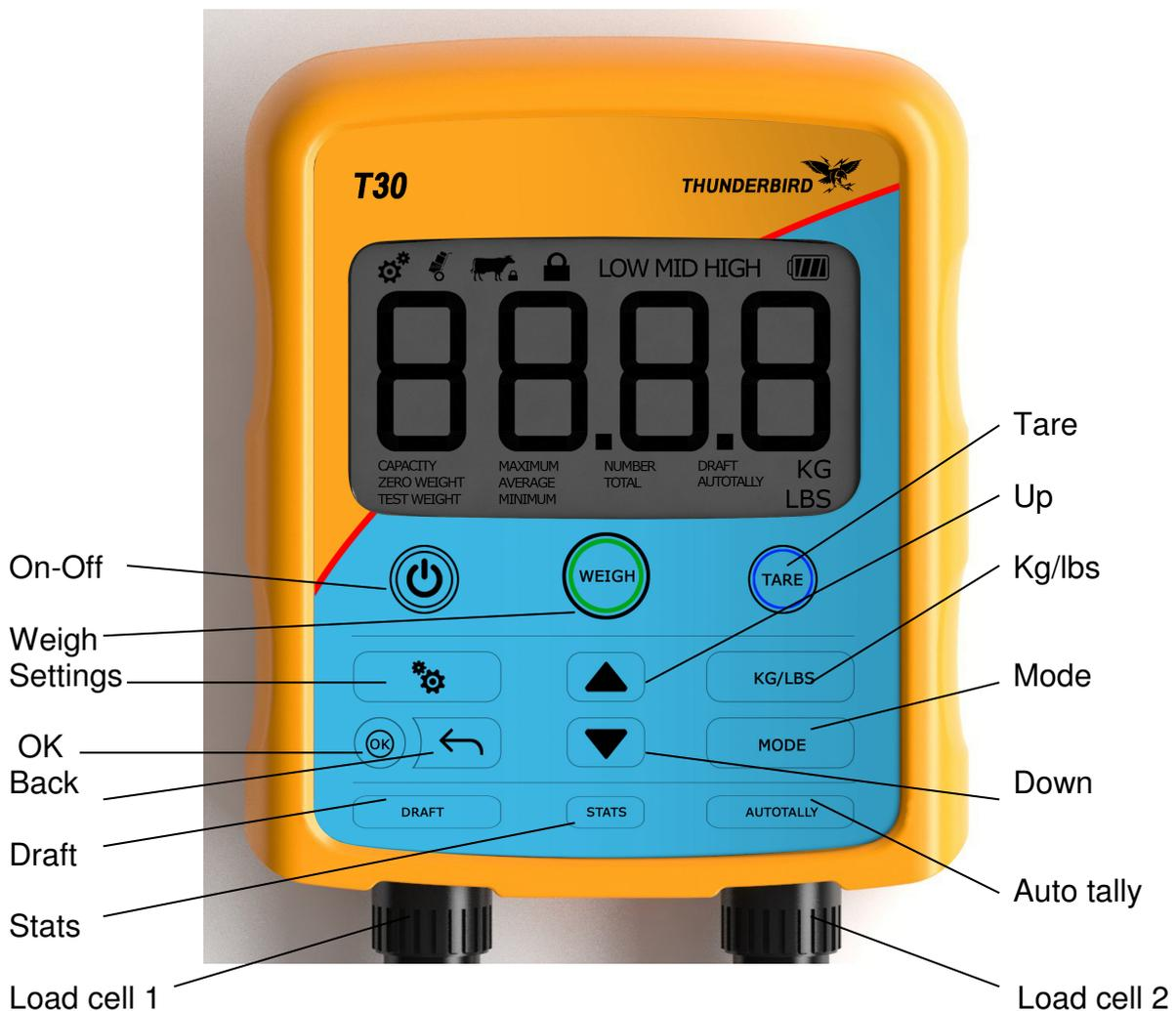
The T30 has a water resistant 13 button keypad for a user interface. An extra large 40mm digit display provides the user with the ability to view the weight at a distance. The display also has other indications that are used at various times. All mode settings and changes are memorized at the time of change, so that the indicator will return to the previous set up when it is turned on.
