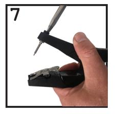
Tighten the nut securely with 8mm socket or screw driver.
