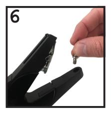
Insert new Junior Combi Pin and attach locking nut.
