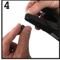
Remove Pin Nut and existing pin from applicator.
