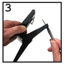
Usin an 8mm socket or a flat head screw driver unscrew existing pin
