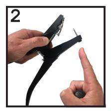
Multi Pins replace pins in both Drovers and Allflex applicators.
