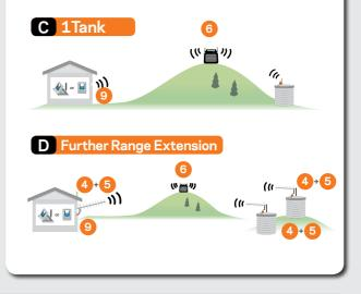
Two base unit systems are needed. One automatically maintains tank level (pump shed to tank) and the other monitors tank level to confirm system is working correctly (tank to house).
