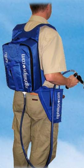
BACKPACK WITH MATERIAL HOLSTER SHOWING CONTAINER IN INVERTED POSITION
