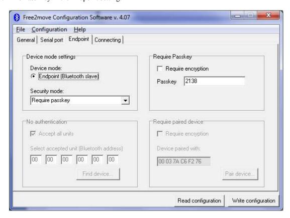
3. Change the Device mode from Slave to Master. Below are the Connecting setting for a master. When you have change it to a Master you can then Pair to a device such as a scale head with built in BlueTooth.
